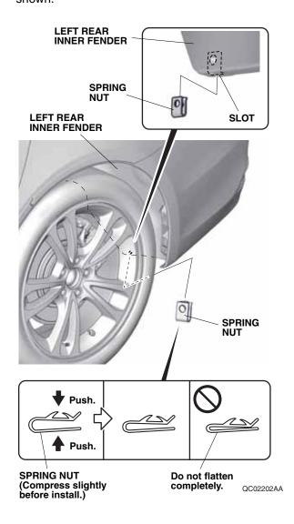
8. Install one spring nut on the left rear splash guard in the direction shown.
