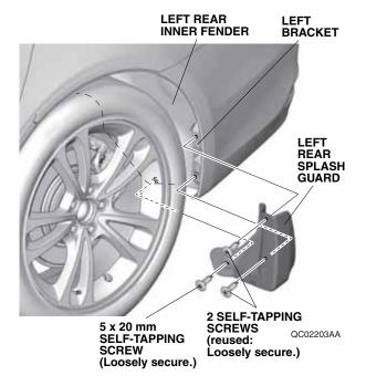
10. Loosely secure the left rear splash guard to the rear bumper with one additional 5 x 20 mm self-tapping screw.
