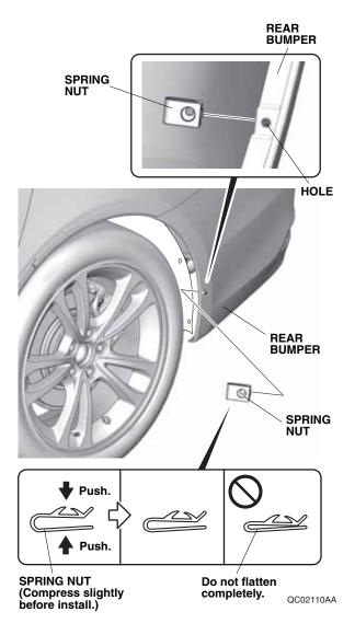
4. Get the left bracket and install two spring nuts on it in the direction shown.
