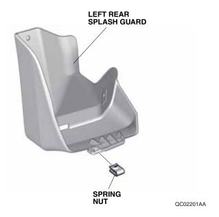
9. Loosely install the left rear splash guard on the left bracket and left rear inner fender with one 5 x 20 mm self-tapping screw and two of the self-tapping screws removed in step 1.
