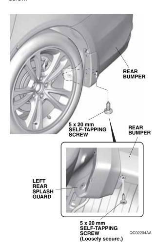
11. While holding the left rear splash guard against the rear bumper, tighten the four self-tapping screws in the order shown.
