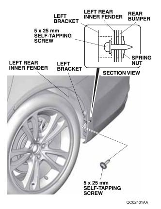
Slightly compress the spring nut. Install one spring nut on the left rear inner fender in the direction shown.
