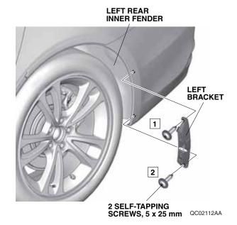
6. Secure the left bracket to the rear bumper using a 5 x 25 mm self-tapping screw. Thread the screw into the spring nut through the left rear inner fender.
